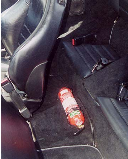
Figure 15 Fire extinguisher fitted to the rear tunnel of a 911
